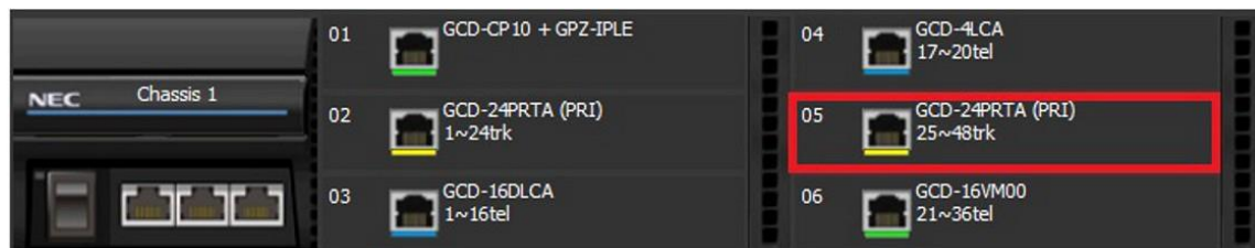
Digital Trunk Clocking Example 2
